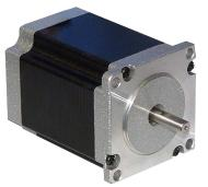
The 23Y310S-LW8-MS High Torque Stepper Motor offers a great value without sacrificing quality. This motor was designed to offer the highest possible torque while minimizing vibration and audible noise. It is wired in series with a Molex 4 pin Mini-Fit Jr. receptacle.
